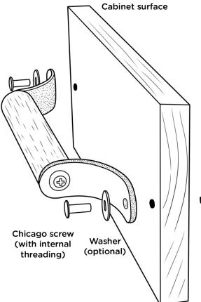
Back screw (different lengths for different cabinet widths)
